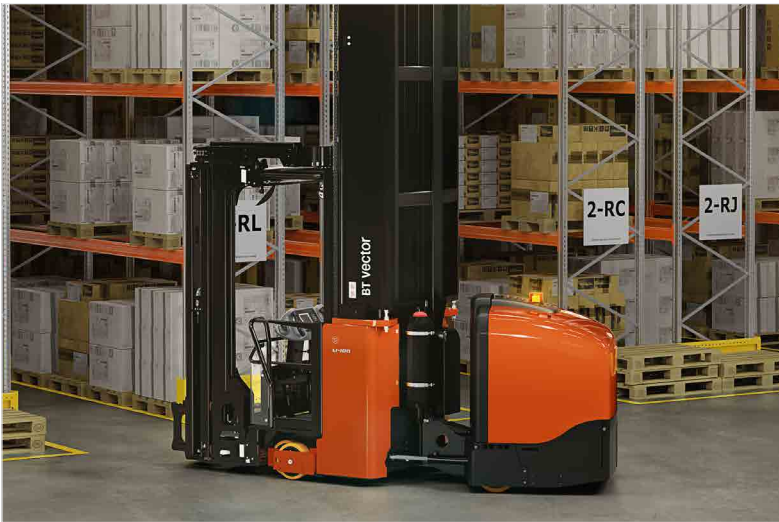
The articulated chassis allows for a more compact turning radius, resulting in saving space and time.
